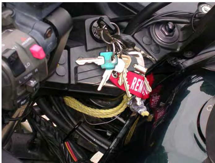
The main fairing stay assembly on the author's Connie is secured with a combination of zip ties, wire and nylon rope.
